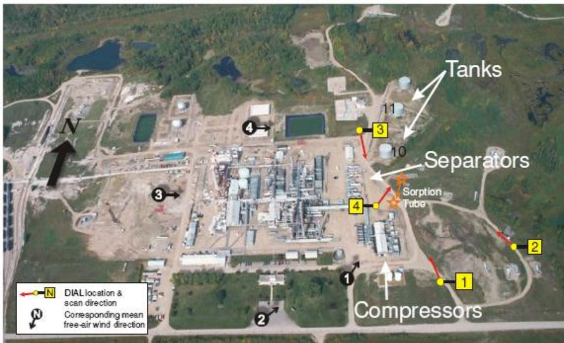
The DIAL technology provided a measure of the overall site emission rate and the emission rate for some of the operational areas for the day of the survey. It did not provide locations of the emitting sources or changes in emitting patterns over time.
